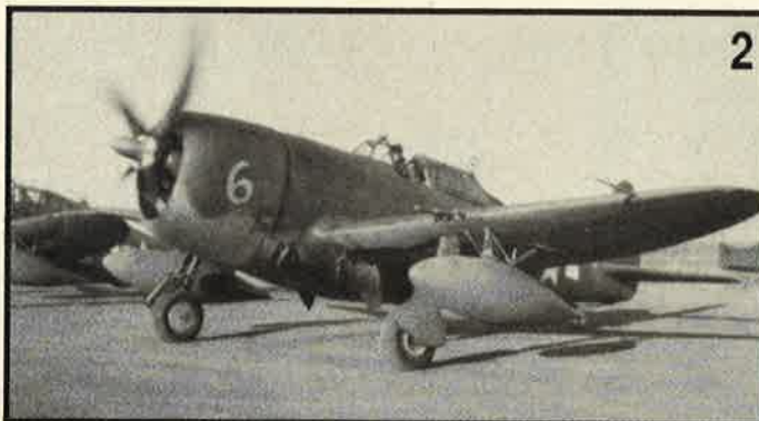
1. During the summer of 1947 fire fighting air drop tests were conducted in Montana by Air Proving Ground and the Forest Service. Stabilizing fins, shown here, were appended to 165-gallon wing tanks, when the P-47 was utilized in a dive bombing mode, which required steep approach in tightly restricted areas, such as narrow canyons. Over generally open areas, the tanks - without fins - were released much like ordinary drop tanks. Of interest is U.S. Forest Service logo on cowl of this P-47N.
