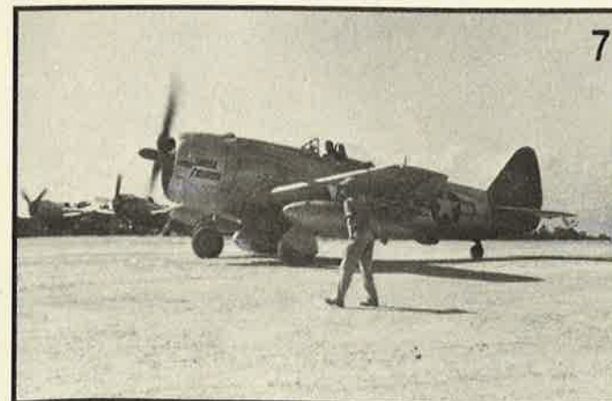
7. Auxiliary fuel tank clearance was minimal for loaded P-47Ns operating out of Ie Shima in August, 1945. Here, Captain Robert Forrest in Shell Pusher revs up to 53 inches of manifold pressure to get off coral strip.
