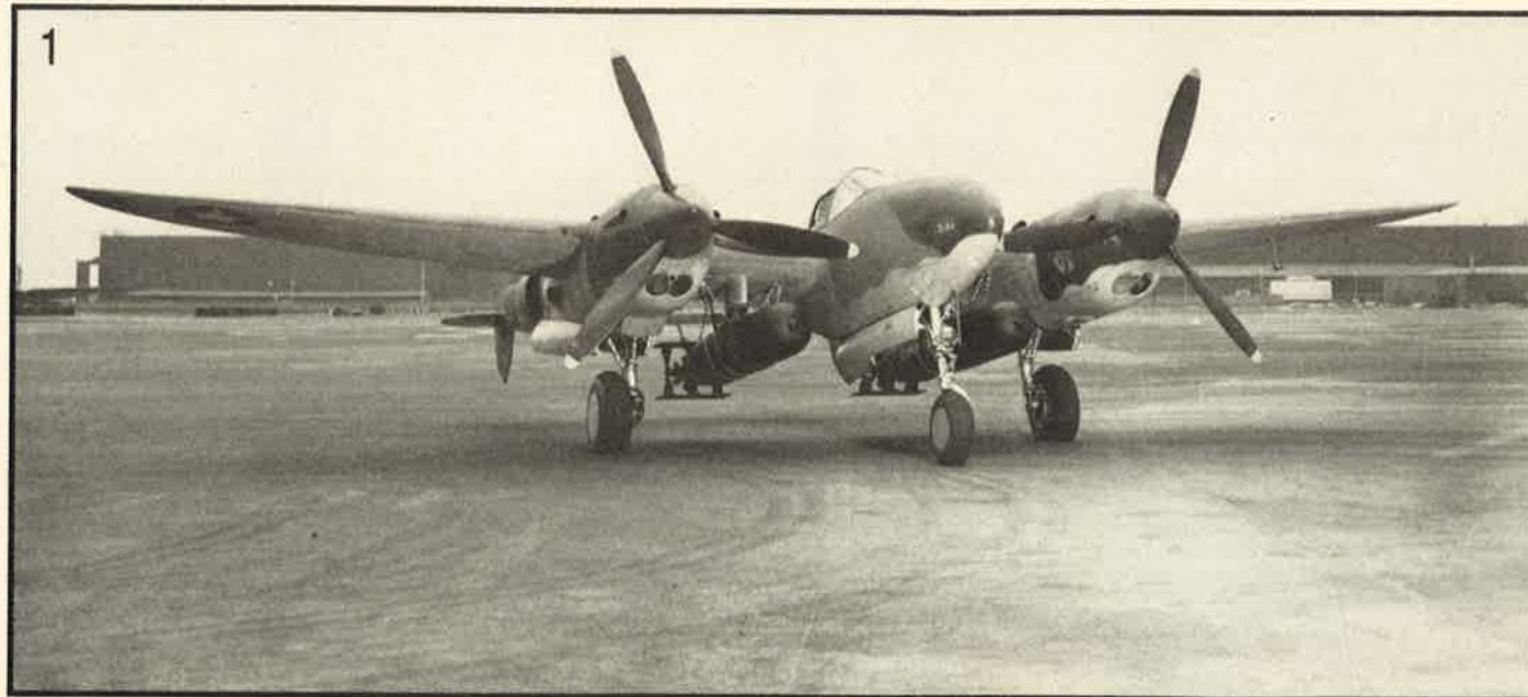
1. Champion U.S. load carrier of WWII was Lockheed P-38 Lightning, but by 1947, when fire fighting tests were run, there were not a great many of them available to the USAF. Lockheed pioneered drop tank pylons and external fuel tanks and was able to attach a great deal of ordnance to their classic twin-engine fighter. Here, a pair of torpedoes on a P-38F.
